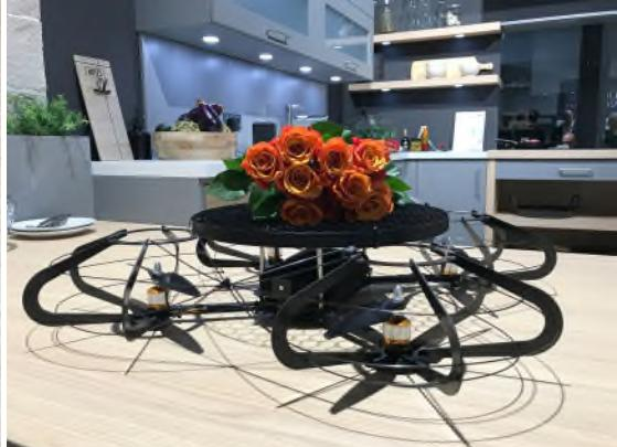
Figure 2: The design of our TrayDrone uses a tray that is designed after an air permeable honeycomb design. Further it comes with designed protectors for protecting the users and the environment from the drone's blades.
