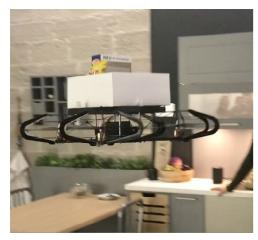
Figure 1: TrayDrone is carrying a box to be delivered to the user in a smart kitchen environment.
