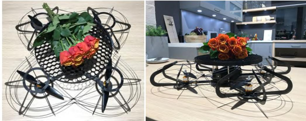
Figure 2: The design of our TrayDrone uses a tray that is designed after an air permeable honeycomb design. Further it comes with designed protectors for protecting the users and the environment from the drone's blades.
