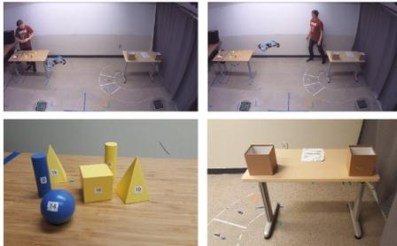
**Figure 1: Top left: The robot doing a supervisory task. Top right: The robot intentionally interferes with the path the user is taking. Bottom: Pick and place task that the user is performing in the videos.**
